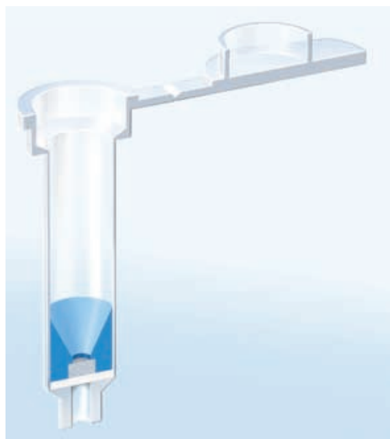
Figure 1: Cross-section view. A reducing device, designed as collecting funnel, creates a cavity for the silica membrane at the bottom of the spin column with a binding capacity of 20 \mu\text{g} . The special design of the blue colored reducing device allows easy central loading of sample and buffer up to 500 \mu\text{l} . Due to the funnel-like design, carry-over contamination is avoided. A foot-hold membrane prevents the silica membrane slipping through the outlet.
